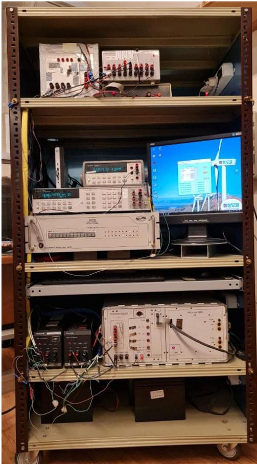
**Fig. 2.** Rack containing all the measurement instruments and sources under test.
