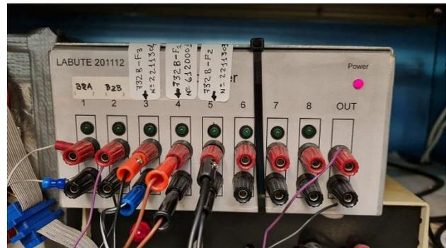
**Fig. 3.** Resistance scanner for temperature measurements.
