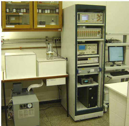
Fig. 2 Primary system of electrolytic conductivity.
